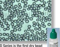
The 4D Series is the first dry bead specifically designed to meet the ISO 21501-4 international standard for improving the repeatability and reproducibility of air particle counters.
